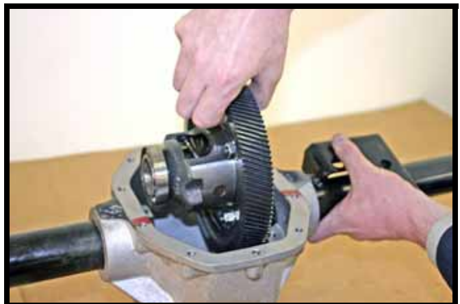
Fig. 14 Removing Differential-Carrier Assembly from Axle Housing
